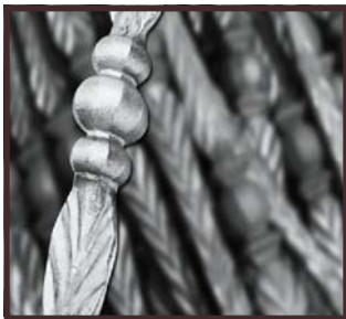
Hot pressed after forging on FG- 139 HFM
